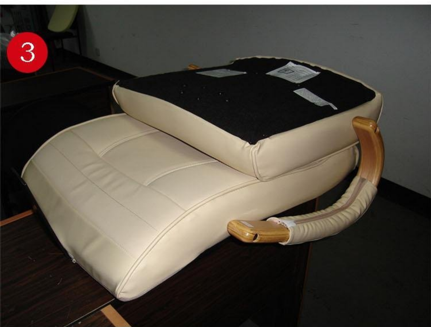
Put the left arm on, but do not tighten the screws
