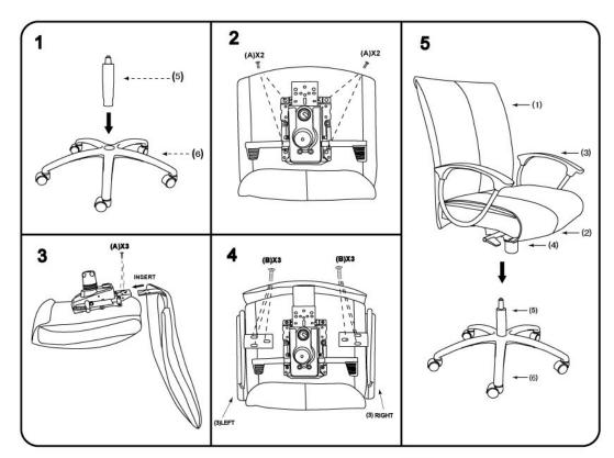
It is important to assemble all parts so that the directional "Arrows" point in the same direction. Make certain that all screws are FULLY tightened before using the chair. Each month, check all screws and tighten any that may have loosend.
