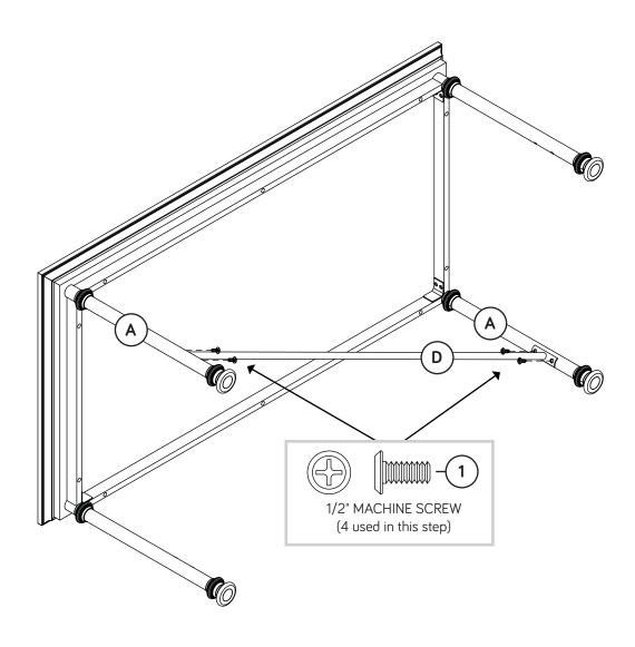
Fasten the remaining END SUPPORT (D) to the ENDS (A). Use four 1/2" MACHINE SCREWS (1).
