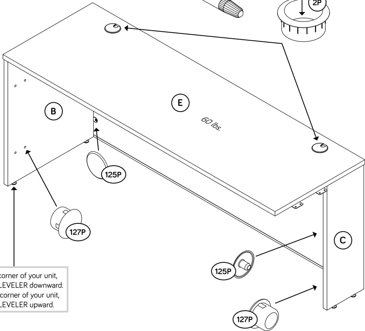
To raise a corner of your unit, rotate the LEVELER downward. To lower a corner of your unit, rotate the LEVELER upward.
