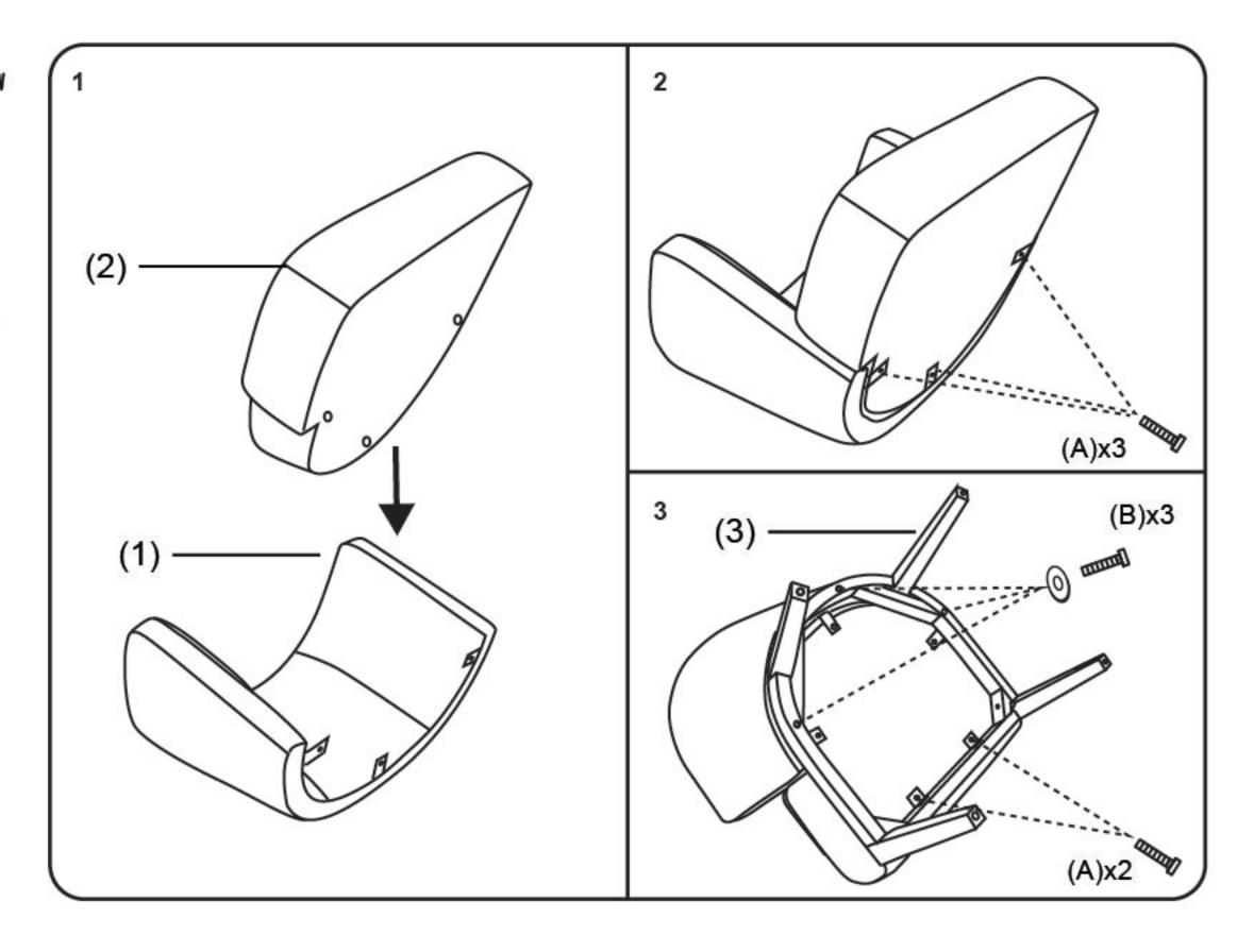
Insert and loosely tighten all screws. When assembly is completed, fully tighten all screws before using. This chair is only intended for sitting. Any other use will void the warranty.
